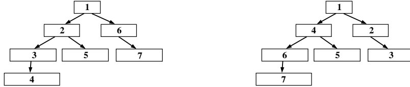
Figure 2.9. In the distributed deployment algorithm of Table 2.6, explorer agents search the partition tree \mathcal{T}_{\mathcal{P}} depth-first for leader or proxy tasks they could perform. An agent in a cell, say c_{\xi} , can always order the gap edges of c_{\xi} , e.g., counterclockwise from the parent gap edge g_{\xi} . The depth-first search progresses by the agent always moving to the next unvisited child or unexplored gap edge in that ordering. The agent thus moves from cell to cell deeper and deeper until a leaf (a vertex with no children) is found. Once at a leaf, the agent backtracks to the most recent vertex with unvisited child or unexplored gap edges and the process continues. As an example, (left) shows the depth-first order an agent would visit the vertices of \mathcal{T}_{\mathcal{P}} in Fig. 2.3f if the gap edges in each cell were ordered counterclockwise from the parent gap edge. If the agent instead uses a gap edge ordering cyclically shifted by one, then (right) shows the different resulting depth-first order. If each agent uses a different gap edge ordering, e.g., cyclically shifted by their UID, then different branches of \mathcal{T}_{\mathcal{P}} are explored in parallel and the deployment tends to cover the environment more quickly.
