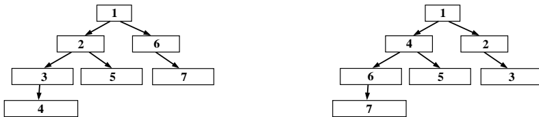
Figure 11. In the distributed deployment algorithm of Table VI, explorer agents search the partition tree \mathcal{T}_{\mathcal{P}} depth-first for leader or proxy tasks they could perform. An agent in a cell, say c_{\xi} , can always order the gap edges of c_{\xi} , e.g., counterclockwise from the parent gap edge. The depth-first search progresses by the explorer agent always moving to the next unvisited child or unexplored gap edge in that ordering. The agent thus moves from cell to cell deeper and deeper until a leaf (a vertex with no children) is found. Once at a leaf, the agent backtracks to the most recent vertex with unvisited child or unexplored gap edges and the process continues. As an example, (left) integers (not to be confused with PTVUIDs) show the depth-first order an agent would visit the vertices of \mathcal{T}_{\mathcal{P}} in Fig. 3f if the gap edges in each cell were ordered counterclockwise from the parent gap edge. If the agent instead uses a gap edge ordering cyclically shifted by one, then (right) shows the different resulting depth-first order. If each agent uses a different gap edge ordering, e.g., cyclically shifted by their UID, then different branches of \mathcal{T}_{\mathcal{P}} are explored in parallel and the deployment tends to cover the environment more quickly. Cf. Fig. 10.
